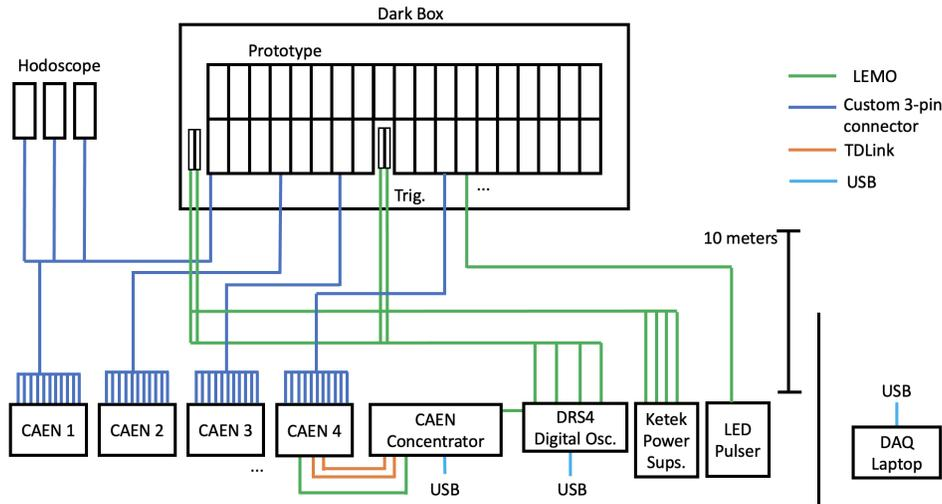
FIG. 8. The DAQ system for the generation 2 CALI prototype at Brookhaven National Lab.
