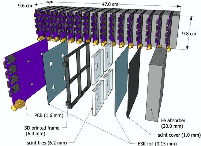
FIG. 2. The SketchUp model of the HCAL insert prototype. Ref. [4]
