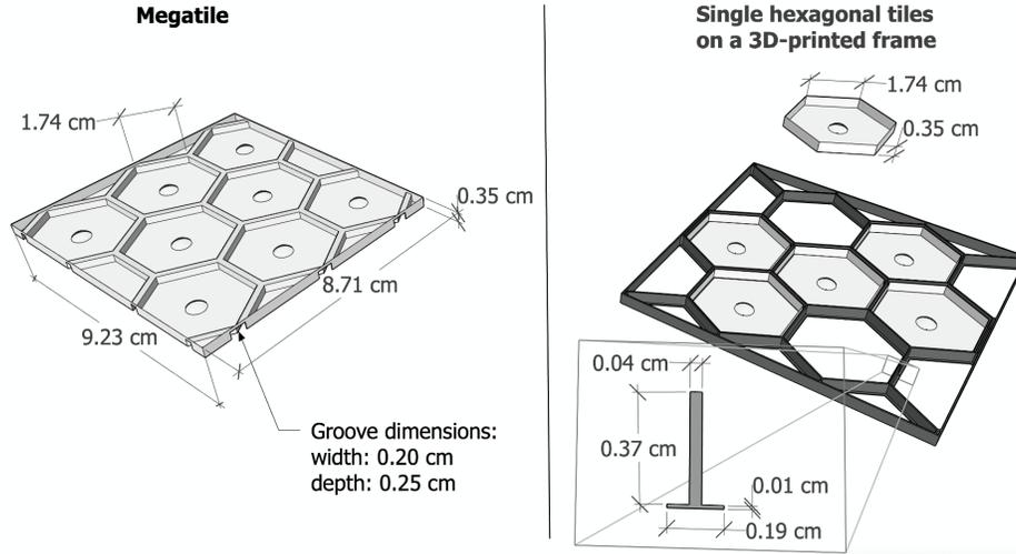
FIG. 1. A render of hexagonal tiles machined within a megatile (left), and hexagonal tiles separated with a 3D printed frame (right). Ref. [3]
