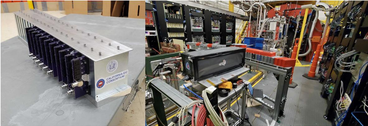
FIG. 3. Photos of the HCAL insert prototype just after assembly (left) and installed in front of the Glue-X experiment at Jefferson Lab (right). Ref. [4]
