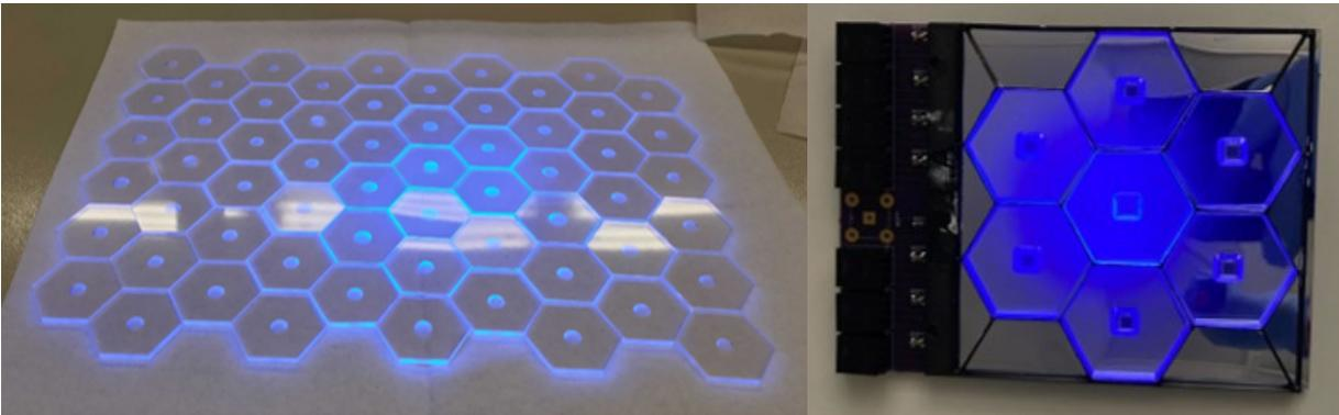
FIG. 7. Hexagonal scintillating tiles machined at UCR (left) and installed in a PCB with reflective foil (right).
