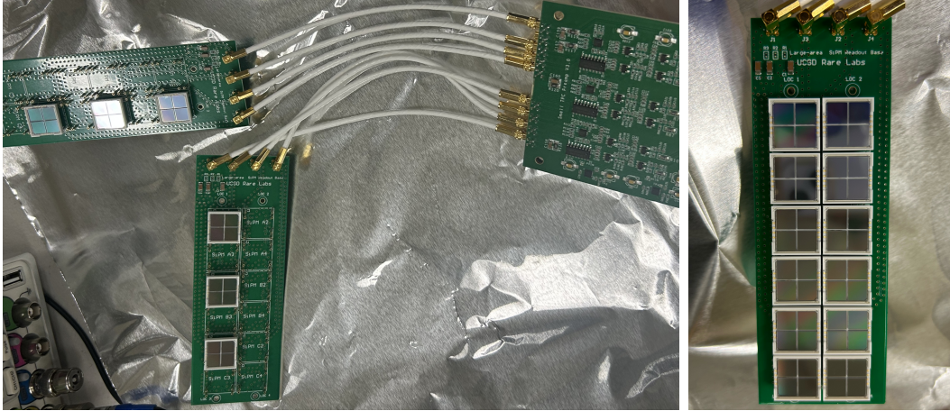
Figure 2.2: Left: First SiPM test configuration. Two baseboard containing three SiPMs were readout individually through a single preamplifier board. All PCB boards were placed inside a cryogenic chamber in order to reduce noise. Right: One baseboard with all 12 SiPMs installed.
