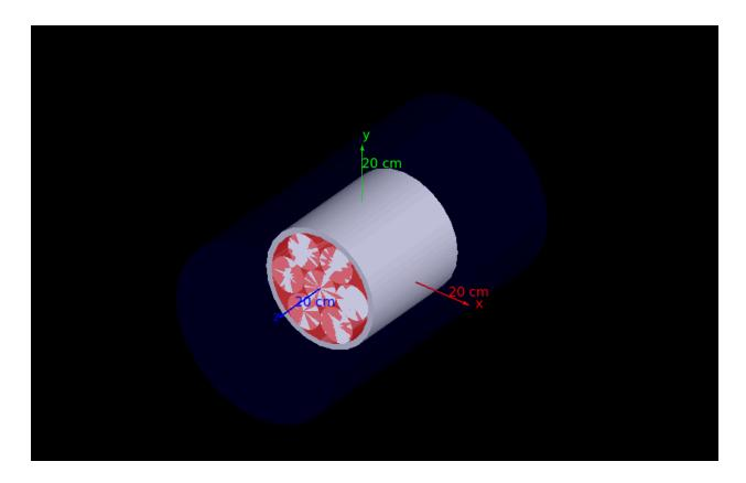
The blue represents a liquid xenon (LXe) bath. The white barrel is a PTFE reflector of xenon light, and the red volume represents the inner LXe volume that will be used to track particle interactions.
